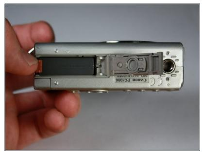
• Pull the orange lever and the battery will spring out slightly.
