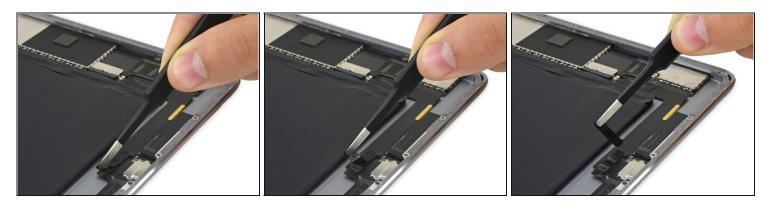
• Remove the tape covering the speaker ZIF connectors.
