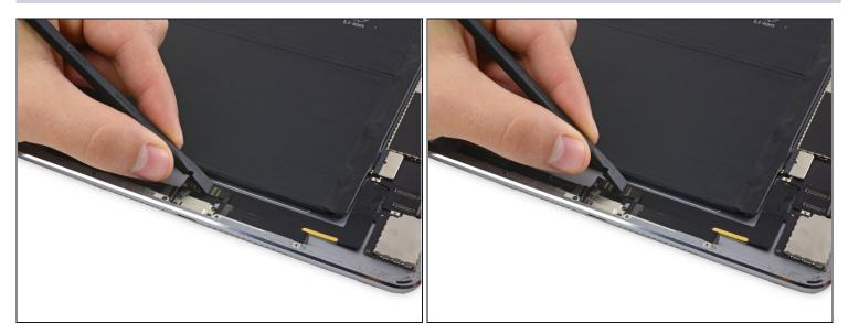
• Use the flat end of a spudger to flip up the retaining flap on the right speaker ZIF connector.
