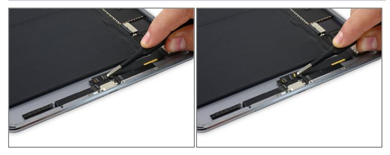
• Slide the speaker cable out from its ZIF connector.
