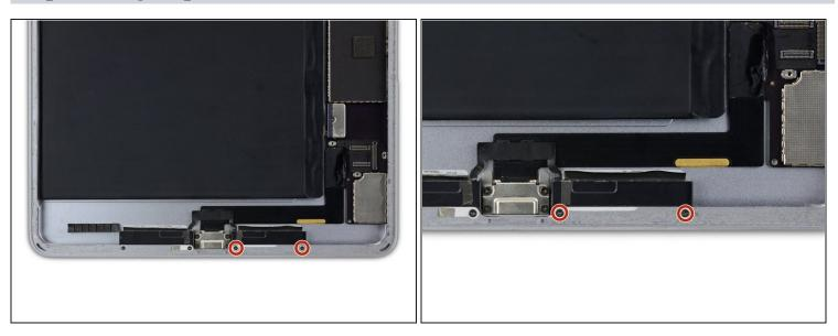
• Remove the two 1.5 mm Phillips #00 screws to the right of the Lightning port.
