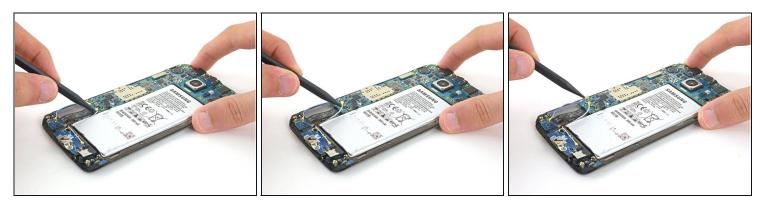
• Use the pointed end of a spudger to disconnect the two antenna interconnect cables from the motherboard.
