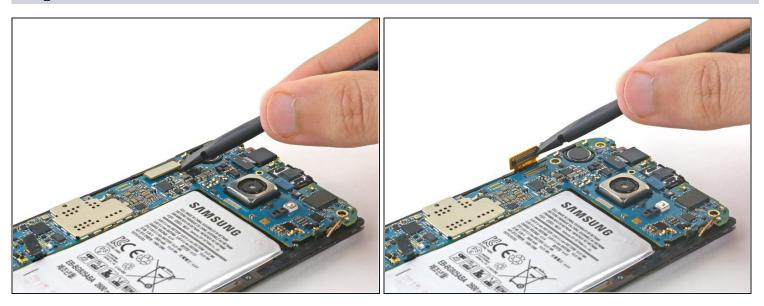
• Disconnect the display ribbon cable from the motherboard using the flat end of the spudger.
