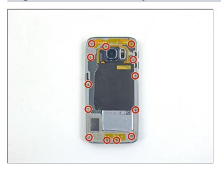
• Remove the thirteen 3.3 mm Phillips #00 screws from the midframe.
