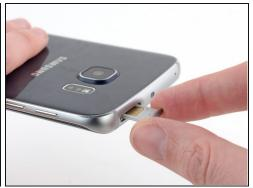
Insert a paper clip or SIM eject tool into the hole in the SIM card slot on top of the phone.
