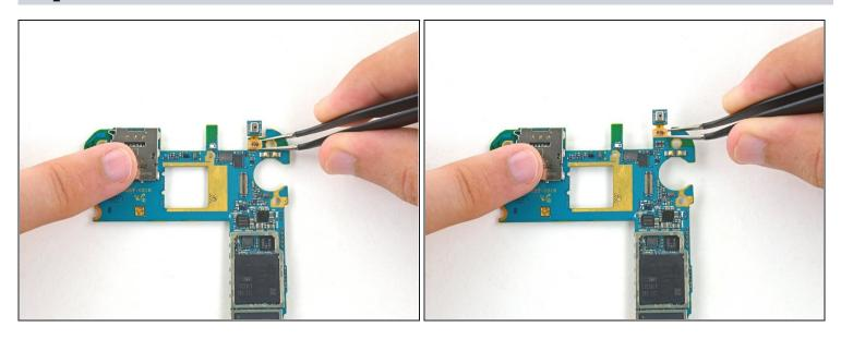
Remove the microphone from the motherboard.
