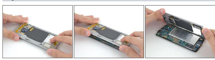
• Press down on the back of the battery and lift up on the edges of the midframe to separate it from the rest of the phone.
