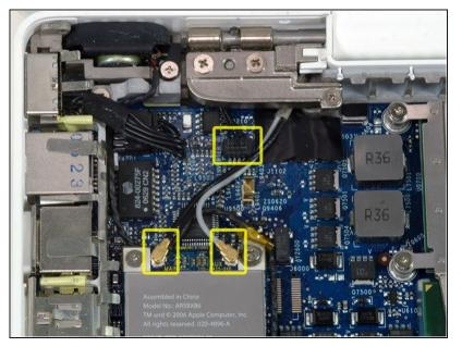
Disconnect the two antenna cables from the Airport card, and the black inverter cable from the logic board. (Pull vertically on all three.)
