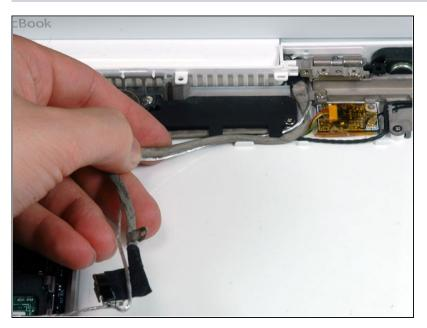
Deroute the silver microphone cable and gray display data cable from the tabs at the bottom of the subwoofer.
