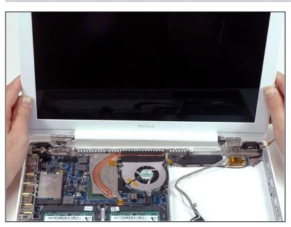
Grasp the display assembly on either side, and lift it up and out of the computer.
