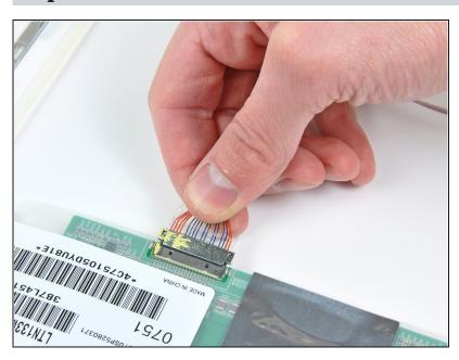
Disconnect the display data cable from the back of the display.
