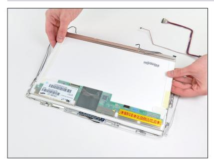
• Lift up the LCD panel by its bottom edge and slide it out of the metal mounting brackets.
