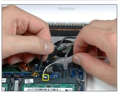
Lift up on the black right speaker cable with one hand, and deroute the silver microphone cable from the silver metal clip just above the right RAM slot.
