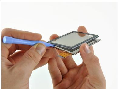
Continue sliding the plastic opening tool along the bottom and up the left edges of the LCD to separate the touchscreen from the LCD.
