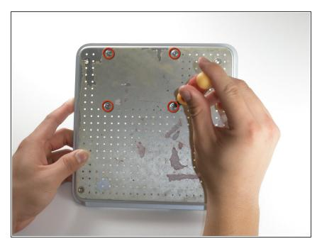
Remove the four T8 Torx screws securing the hard drive to the lower case.
