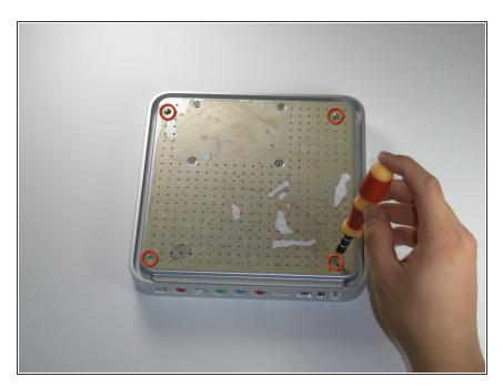
Remove the four T10 Torx screws that secure the lower case to the upper case.
