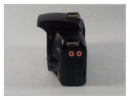
Remove the two 3mm (1/8") black screws from the side cover using a #00 Phillips screwdriver.
