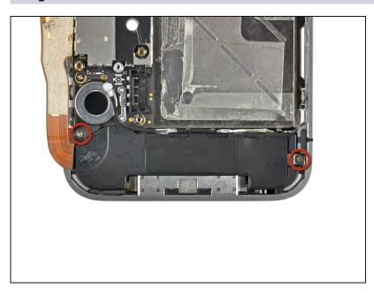
• Remove the two 2.4 mm Phillips screws securing the speaker enclosure assembly to the outer case.
