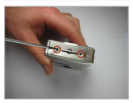
Remove screws on strap panel of camera.
