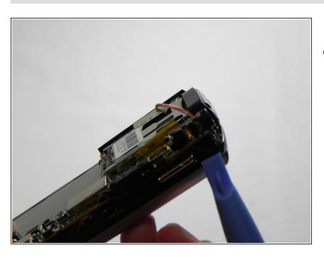
Next, use a plastic removal tool and separate the silver front case from the black frame.
