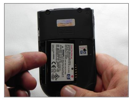
Now, lift the battery up and away from the device to remove it.
