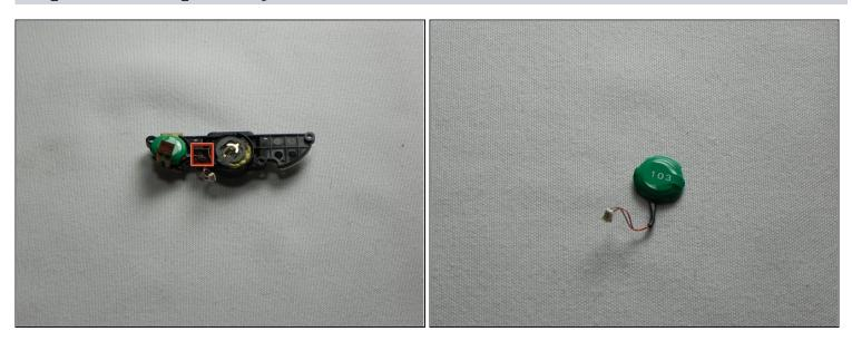
• once the joypad key have been removed use the <u>tweezers</u> to carefully maneuver the wire out of its clip releasing the battery
