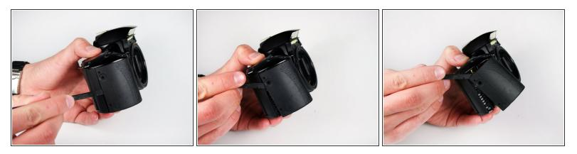
• Use the spudger tool to carefully pry the grip from the rest of the camera.
