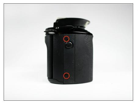
Remove the two 4.5mm (.18in) long black screws from the camera grip using a #00 Phillips screwdriver.
