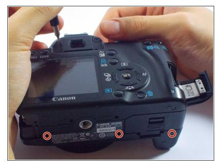
Remove three medium length screws from the bottom of the camera
