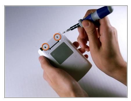
Unscrew the two 7.35mm Torx T6 screws.
