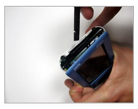
Using the flat end of the spudger, carefully pry the black cover on the top from the blue front cover.
