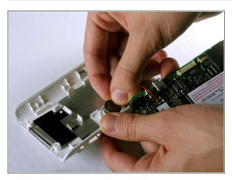
Carefully remove the speaker from the back white cover by just pulling it gently. It is glued on.
