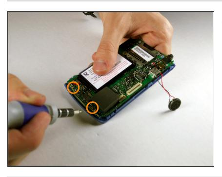
Unscrew the #00 5.75mm Phillips screws from the bottom of the motherboard. The front blue panel should fall right off.
