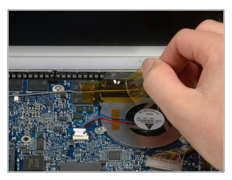
Peel up the orange Kapton tape securing the right speaker cables above the right fan.
