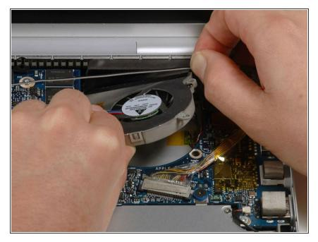
Hold up the gray and black speaker cable with one hand. Use your other hand to lift the right fan up and carefully peel up the tape securing the fan to the heat sink as you go.
