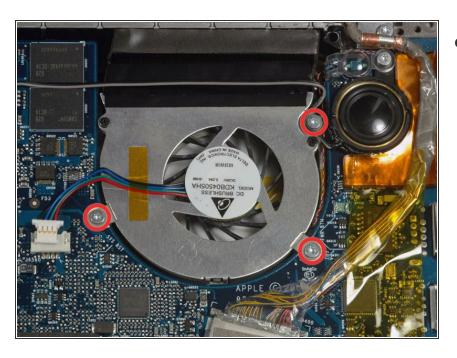
Remove the three silver T6 Torx screws securing the right fan to the logic board and lower case.
