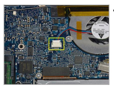
Disconnect the right fan cable from the logic board.
