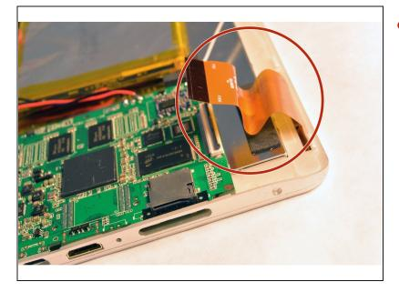
• Open the ZIF connector. Then, remove the ribbon that connects the motherboard and the screen.
