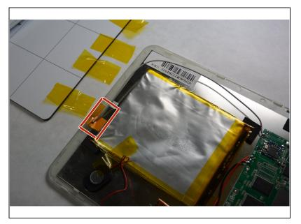
• Disconnect the Wi-Fi antenna cable from the motherboard.
