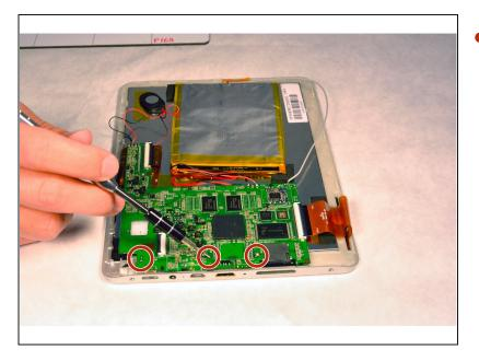
• Using the Phillips #1 screwdriver, remove the three screws from the motherboard..
