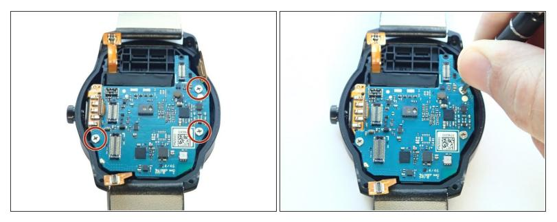
Remove three 3.0 mm Phillips screws on the edges of the motherboard with a Phillips #000 screwdriver.
