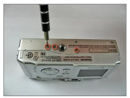
Use the Phillips #00 screwdriver to remove the three 2.8 mm screws on the bottom of the camera.
