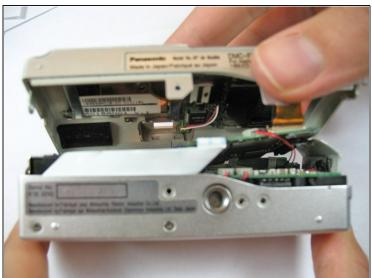
$\triangle$  Be careful not to damage the ribbon cable when opening. Ensure it is still attached.
