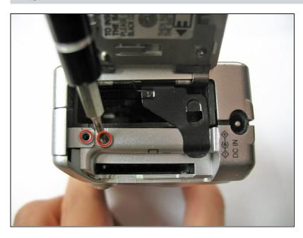
Using the Phillips #00 screwdriver, remove the two 2.8 mm screws located under the hatch.
