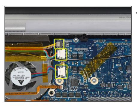
Disconnect the iSight, inverter, and left fan cables from the logic board.
