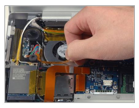
Peel up the left ambient light sensor cable from above the left fan.
