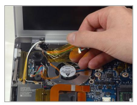
Peel up the iSight and inverter cables from above the left fan, removing tape as necessary.
