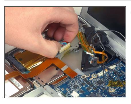
Disconnect the large multi-colored power cable from the left I/O board.
