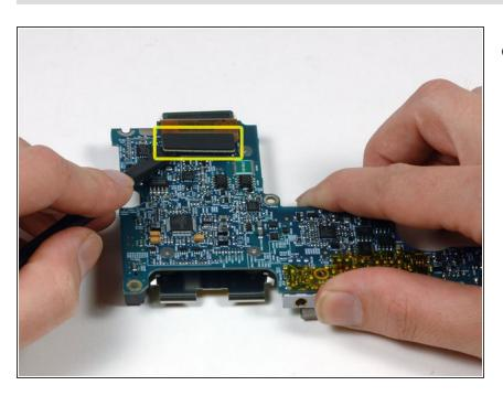
Turn the left I/O board over and disconnect the short left I/O board cable.
