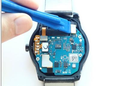
• With a plastic opening tool, disconnect the four connectors on the top of the motherboard.
