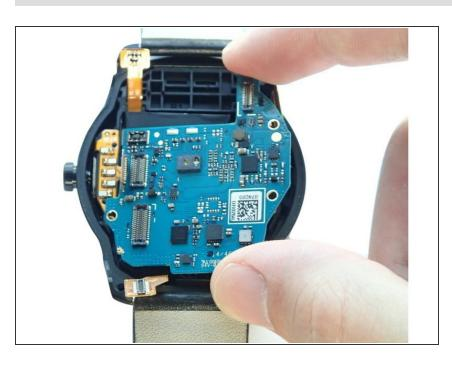
Grasp the edges of the motherboard and slide it slightly towards the right to remove it from its case.
