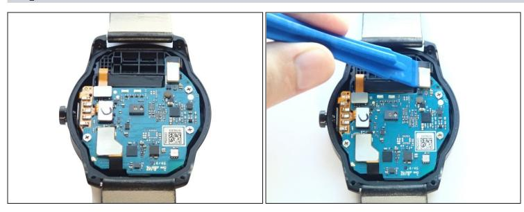
• With a plastic opening tool, disconnect the four connectors on the top of the motherboard.
