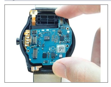
Grasp the edges of the motherboard and slide it slightly towards the right to remove it from its case.
