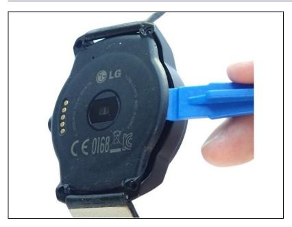
Use a plastic opening tool to pry open the back case from both sides of the watch.
