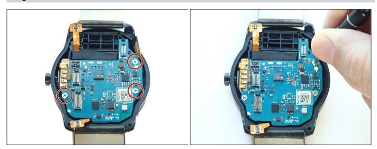
• Remove three 3.0 mm Phillips screws on the edges of the motherboard with a Phillips #000 screwdriver.
