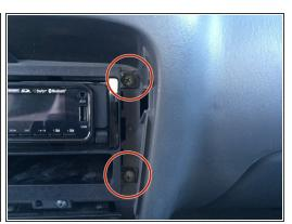
• Once the trim is removed, remove the four screws found on each corner of the stereo.
