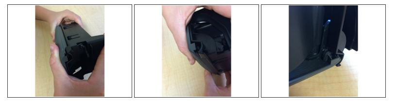
• Check to see if the broken parts of the cup holder have stayed connected by the glue, by pressing them together for about 2 minutes
