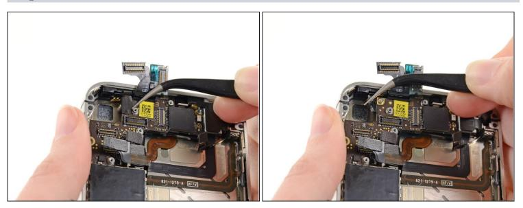
(i) If present, remove the piece of tape covering a Phillips screw near the power button.
