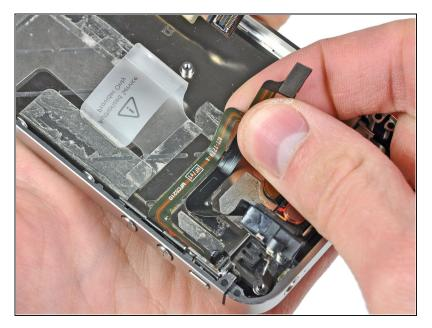
Carefully peel the headphone jack/volume button cables off the adhesive securing them to the rear case.
