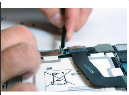
• Using the spudger, disconnect the charge port from the motherboard.
