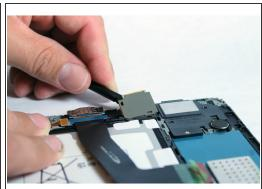
Using the spudger, pry out the SD card slot.
