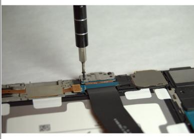
Remove the two 2 mm Phillips #000 screws in the charge port bracket.
