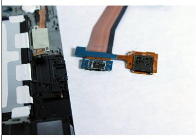
Pull out the charge port and the SD card slot.
