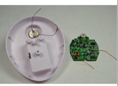
Unsolder the red cables from the metal plates.
