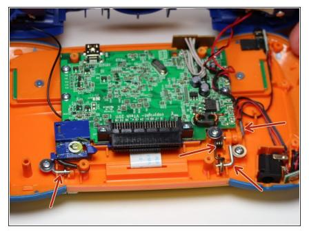
• Remove the three "L" shaped brackets and the spring.
