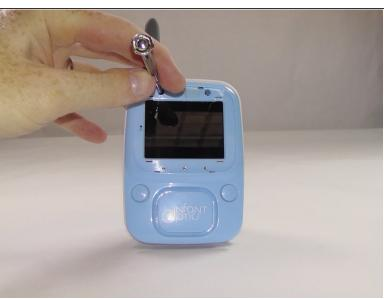
Using a Phillips #2 screwdriver, remove the two 6.0 mm Phillips screws that are exposed after removing the face plate.
