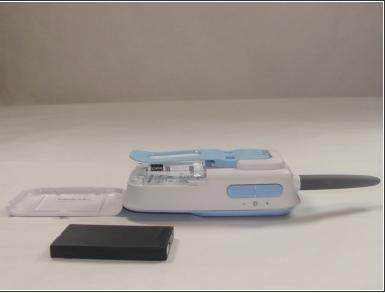
Remove the battery by pushing in on the right side and then pulling the battery up and out of the body of the hand held monitor.
