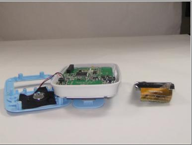
Remove the hand held monitor screen from the mother board by carefully pulling from the point where it is attached with an adhesive to the mother board. To reassemble your device, follow these instructions in reverse order.
