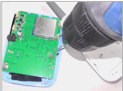
• Using a drill carefully drill out the plastic posts that connect the mother board to the face plate.
