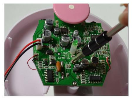
• Remove the 7mm Phillips #1 screw in the middle of the motherboard.
