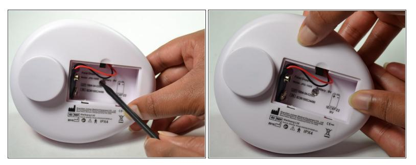
• Puncture the sticker in the battery compartment with a spudger to access the screw beneath it.
