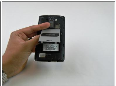
Place the plastic opening tool at the bottom edge of the battery and lift up. Carefully remove battery with your hands.
