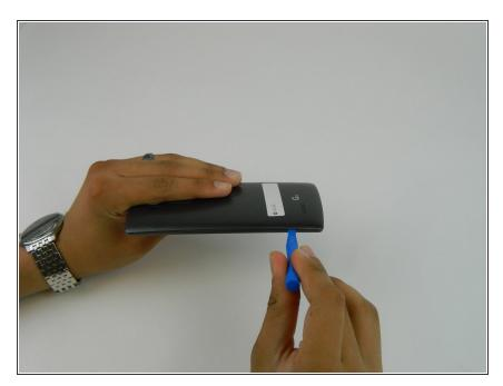
First, make sure the phone is powered off. Remove the rear cover by placing the plastic opening tool in the groove on the bottom left side of the LG G4 and gently prying up.
