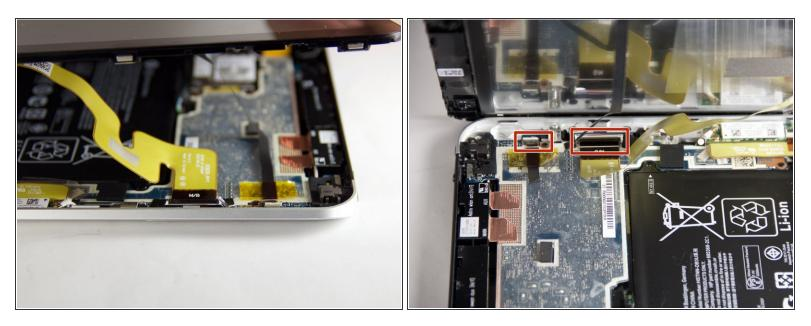
Use the tip of a spudger to disconnect the two display <u>ZIF connectors</u>.
