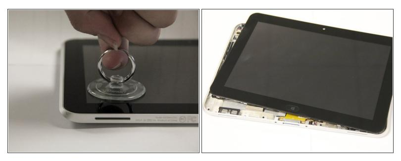
• Use a suction cup to pull the display assembly up.
