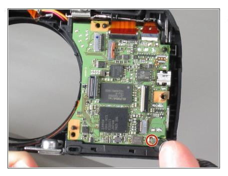
Remove 1-2.5 mm screw using a Phillips #000 screwdriver.
