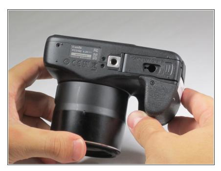
Using your fingers, slide the battery compartment door to the right until it unlocks.
