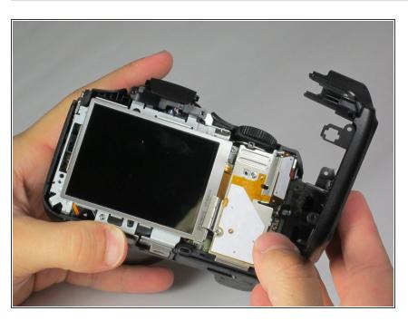
Once all screws are removed, pull the back facing off with your fingers.
