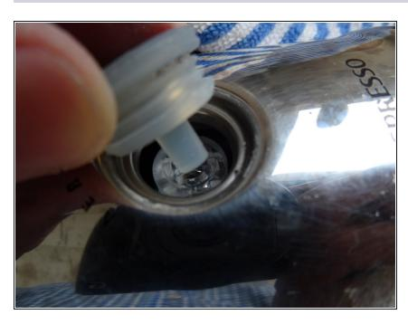
Carefully embed the thermal contact in conducting paste. Then press bottom into body until you hear a clic three times. At last switch must be pressed in. To proof the function use water.
