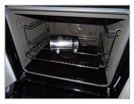
Heat up to 50°C/120°F in oven in order to make the clips inside smooth.
