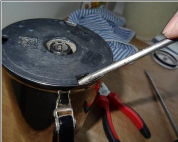
• Open the bottom with a strong screwdriver. Be careful not to break the clips inside
