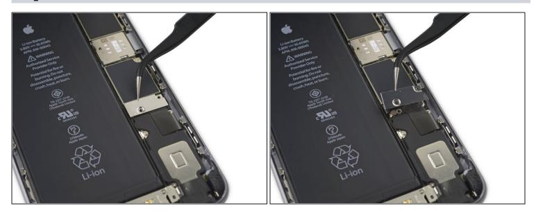
• Remove the battery connector bracket.
