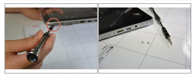
Remove the two screws from the end of the device where the ports are located using a Phillips #1 screwdriver.
