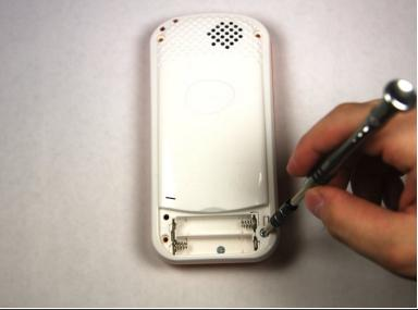
• Remove four 13.8mm screws from the back of the device using a Phillips #1 screwdriver.
