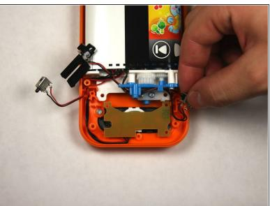
Remove the two buttons, noting how wires are placed for reassembly.
