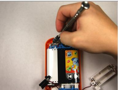
Remove four 7.5mm screws with a Phillips #0 screwdriver.
