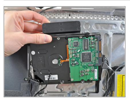
Lift the hard drive off its bottom retaining posts and remove it from the iMac.
