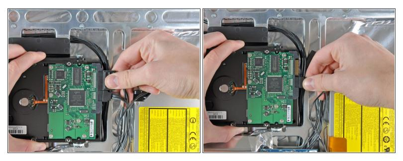
• Disconnect the SATA data and power cables by pulling their connectors away from the hard drive.
