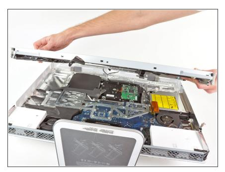
Remove the display assembly from the iMac.
