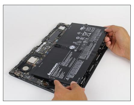
• Carefully lift and remove the battery.
