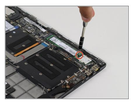
Remove the 1.5 mm screw using the Philips 00 screwdriver.
