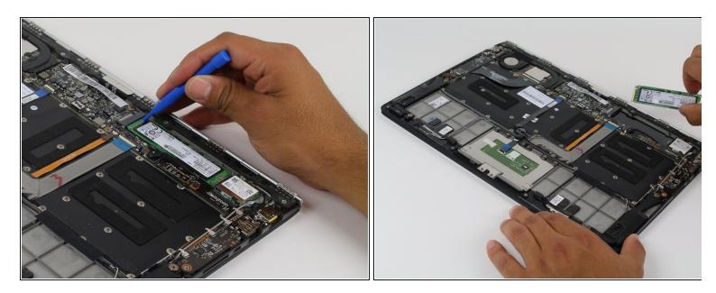
Use the plastic opening tool to remove the hard drive/SSD.
