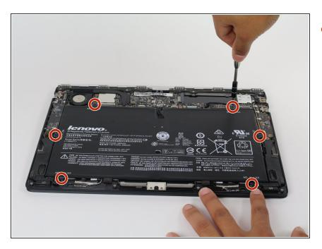
Remove the six 3.5 mm screws surrounding the battery using a Phillips 00 screwdriver.
