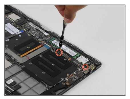
On the other side of the laptop, remove the two 3.5 mm screws using the Philips 00 screwdriver.
