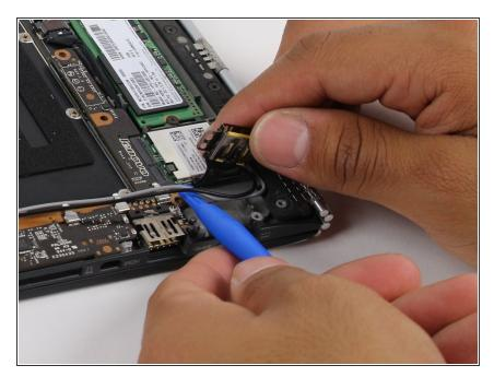
• Lift the USB port up and use the plastic opening tool to loop the wires around the USB port.
