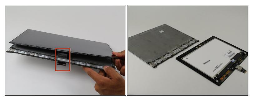
• Unclip the display assembly by sliding the display down, towards the lower edge of the upper case component. The clips will disengage and you will be able to lift the assembly out easily.
