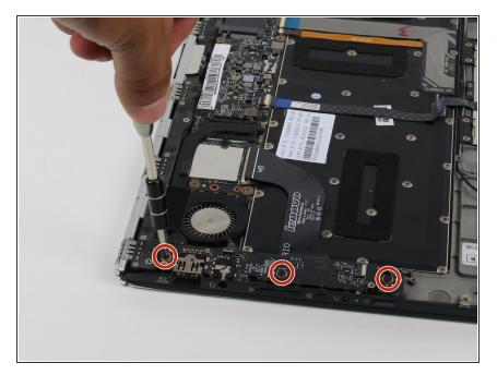
Remove the three indicated 3.5 mm screws using the Philips 00 screwdriver.
