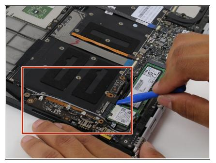
• Remove the USB assembly using the plastic opening tool.
