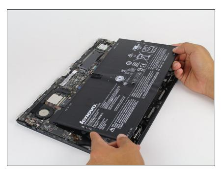
• Carefully lift and remove the battery.
