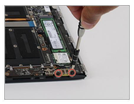
• Remove the two 2.5 mm screws using the Philips 00 screwdriver.
