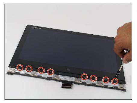
Remove the eight 2mm screws using the Philips 00 screw driver.
