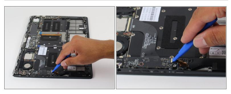
• Using the plastic opening tool, flip open tab as shown.
