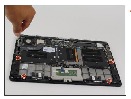
Remove the four 4 mm screws using the Phillips 00 screwdriver.
