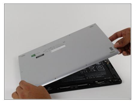
• Remove the panel and place it in a safe location.
