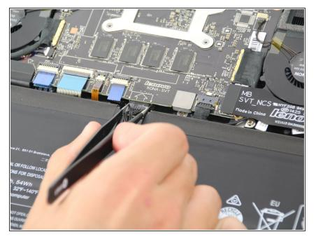
Using either tweezers or your fingers, disconnect the black battery cable by pinching either side of the connector and pulling towards the battery.
