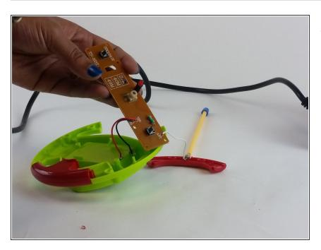
Lift the motherboard to separate it from the remote control.
