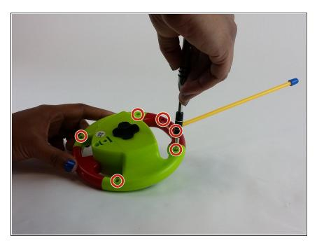
Hold the remote control with the backside facing you and, using the Phillips #00 screwdriver, unscrew the six 6.5 mm screws on the back of the controller that hold it together.
