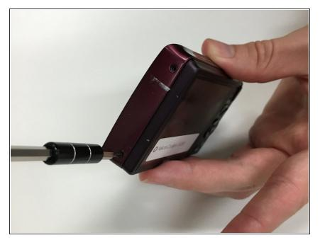
Remove the two 0.1 mm screws using a Phillips Head screwdriver in order to properly open the camera
