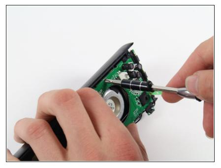
• With the Phillips #2 screwdriver, unscrew the 9.9 mm screw from the larger circuit board surrounding the speaker.
