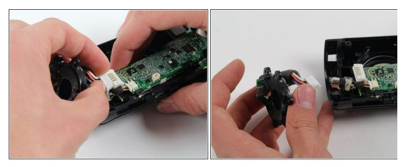
• Finally, after opening the speaker, locate the USB plate on the left face of the speaker and remove it from the motherboard.
