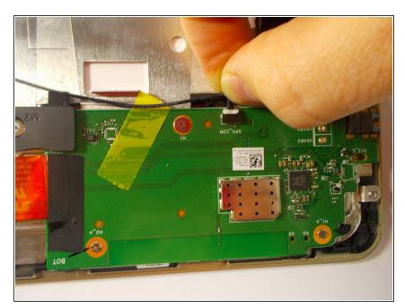
• Remove the tape and unplug the wire that is connected to both of the speakers.
