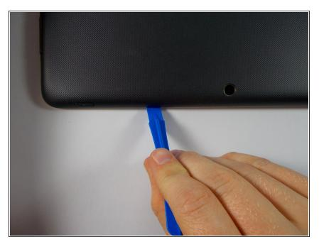
Slide the tool around all four sides of the tablet while gently pulling the tool up.
