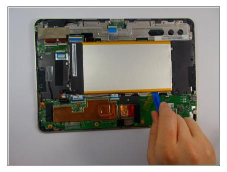
Use the plastic opening tool to carefully pry the battery out from the frame.
