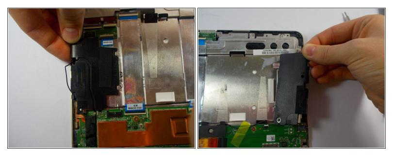
• Remove the two speakers from the frame.
