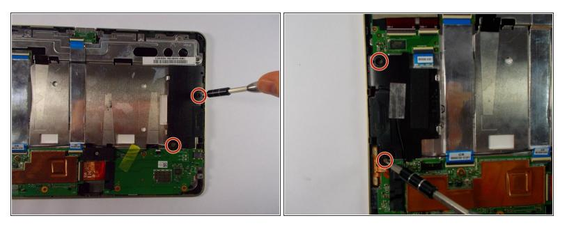
Use the JIS #000 screwdriver to remove the four screws.
