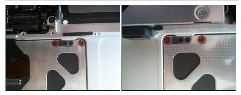
• Remove the four 1.2mm #00 Phillips head screws from rear of the trackpad.
