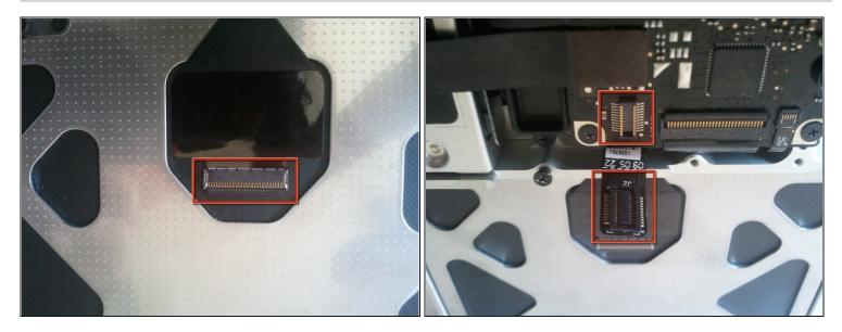
• Remove the ribbon cable by releasing it from the ZIF connector on the underside of the trackpad and also from the socket that attaches it to the logic board.
