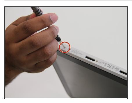
Use a Phillips #000 screwdriver to remove the four 3mm screws.
