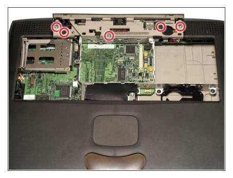
Remove the three long silver and two short black Torx screws from the beige plastic casing.
