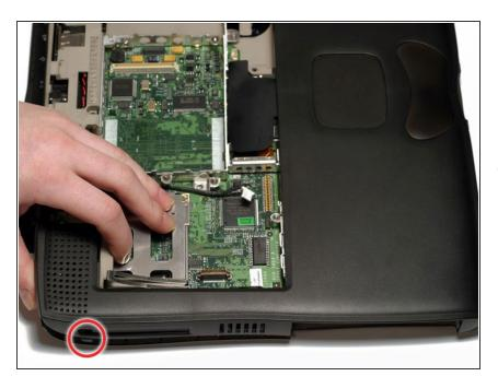
The PC card eject button on the laptop's left side prevents the upper casing from lifting up. In order to bypass the button, push it in far enough so that you can pull the upper casing's left side out and up beyond the button.
