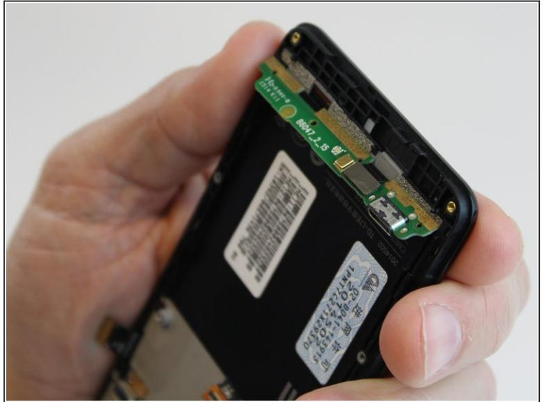
**⚠** Do not remove the PCB circuit board at this time.
