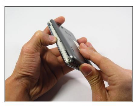
Remove rear battery cover and battery.
