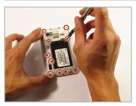
Remove the 10 screws on the rear case.
