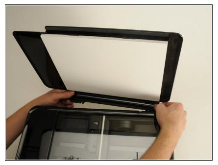
Remove the flap for the scanner.
