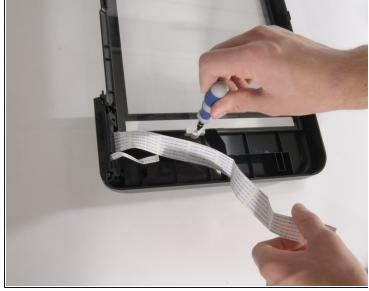
• The scanner glass is held down by one T-9 screw. Use a screw driver to remove the screw.
