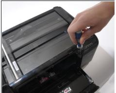
Remove the three screws from the top of the printer with a T-9 screwdriver as shown.
